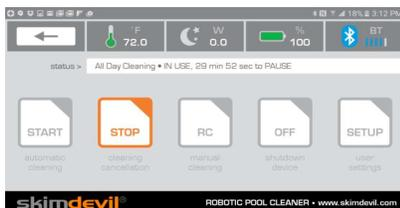
Here you can see that robot is performing All Day Cleaning, is in use, and 29min and 52 sec left to the Pause. By pressing STOP button, the cleaning process will be terminated the App screen will go back to previous picture.
