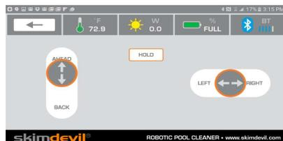
You can control the speed forward and backwards and set it steady by activating HOLD button. With the right hand button you can control the left and right directions. This feature can be used to access specific pool areas for spot cleaning and can offer great fun and entertainment for the whole family.
