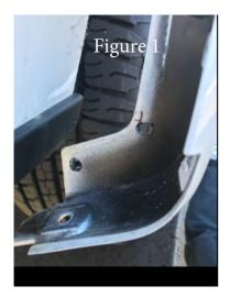
**NOTE**: *Drilling mounting holes in flaps is required for installation.*
