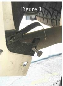
**STEP 2**-Place U-Clips over holes at factory hole locations
