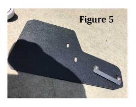
**STEP 3-**Align Mud Flap to your desired positioning to determine the location of the Clamping support Bracket.
