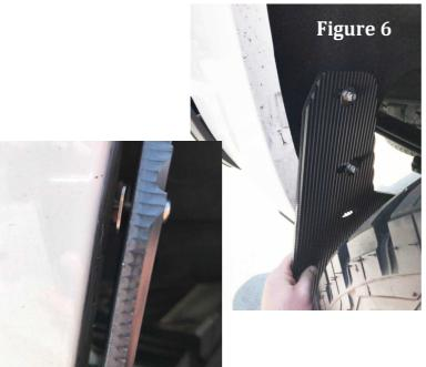
**STEP 5-**With all 4 mounting bolts in place, place a ball of clay or putty on the bolt heads and bolt studs.
