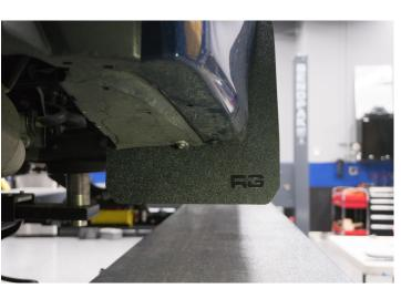
Check flap alignment prior to tightening fasteners
