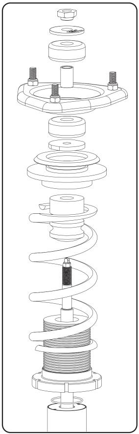
REMOVE OEM SHAFT SPACER BY PLACING SHOCK UPSIDE DOWN IN BENCH VICE. PLACE OPEN END OF 14mm WRENCH ON SPACER AND LIGHTLY TAP WITH HAMMER
