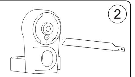
CUT THROUGH BUSHING TO REMOVE FROM TRAILING ARM. BE SURE NOT TO DAMAGE THE HOUSING
