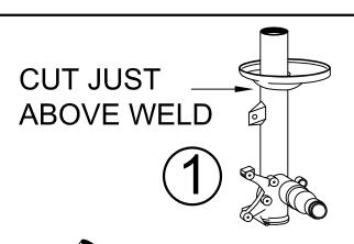
REMOVE STOCK SPRING PERCH BY CUTTING THROUGH THE HOUSING.
