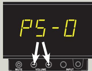
*While flashing, the Volume Up or Down buttons set the PS number. After adjustment, the setting is stored when the display turns off.*
