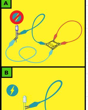
Electricity will alway take the path of least resistance. For example, if you connect the components like in diagram A, the light will not turn on!
