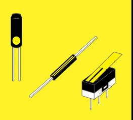
A sensor senses an external pressure or force and sends a signal. Switches are also sensors. The switches in your kit are used as sensors in the everyday world:
