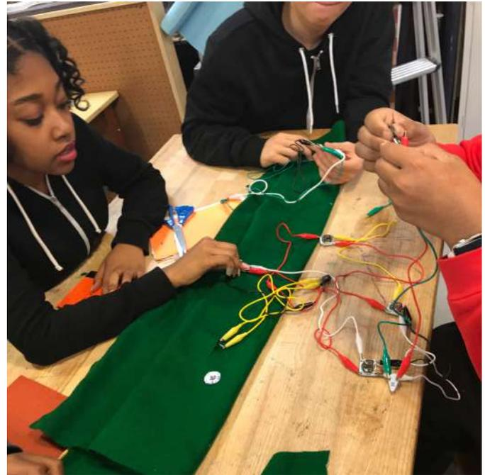
Students at NYSCI are creating circuits using LEDs and the light sensor board and testing them out with alligator clips
