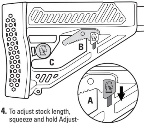
4. To adjust stock length, squeeze and hold Adjust-ment Lever (B). Slide rear portion of stock to desired length and release lever. Rear-stock will automatically engage at the nearest corresponding position. To ensure pin engagement prior to shooting, push or pull on rear portion of stock.
