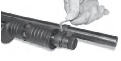
**3** Unscrew the capture screw on the end of the magazine tube (A) and remove the barrel by pulling it out of the receiver (B).
