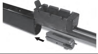
**4** Slide action bar and forend assembly back onto magazine tube. Align action bars with corresponding slots in receiver. (A) Align the follower assembly keeper slot with the opening in the top of the mag tube. (B) Insert the follower assembly keeper through the hole in the mag tube and into the corresponding slot in the follower assembly and forend.
