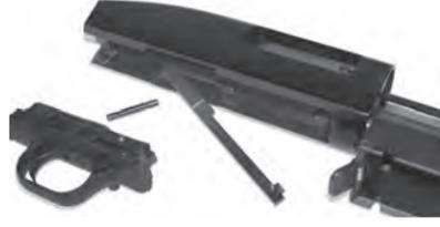
**7** Position the bolt carrier as shown and remove it from the receiver.
