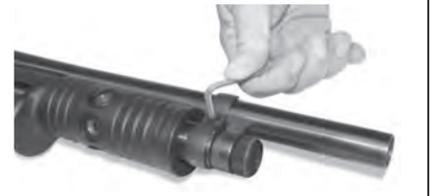
**11** Reinstall stock by aligning front of stock with rear of receiver and utilizing the correct tool re-attach the stock to the receiver. **Note:** Carefully align and position stock prior to tightening in order to avoid stripping threads in the receiver
