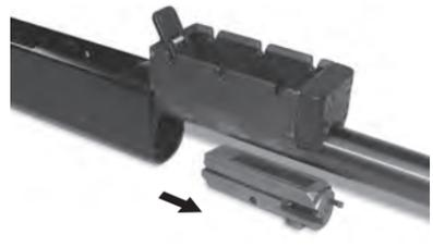
**10** Remove shell lifter from receiver. Shell lifter is held in position by spring tension into corresponding holes in receiver. Squeeze ends to relieve tension for removal.
