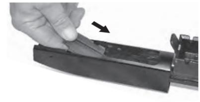
**6** Reinstall left shell stop into corresponding slot in receiver. Hold in position during Step 7.
