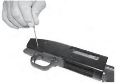
**5** Remove the trigger group rear end first from the receiver. Once the trigger group has been removed DO NOT PULL THE TRIGGER. Serious damage to the trigger group may result.
