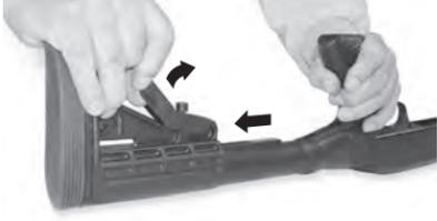
b. Insert 1/4" extended ball end Allen wrench into hole located on bottom of stock. Engage wrench with corresponding mounting bolt and turn counter clockwise until stock is free from rear of shotgun receiver.
