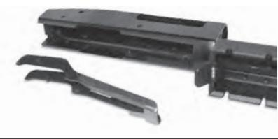
**11** Tip shotgun receiver at a sharp angle to remove follower assembly from inside magazine tube.
