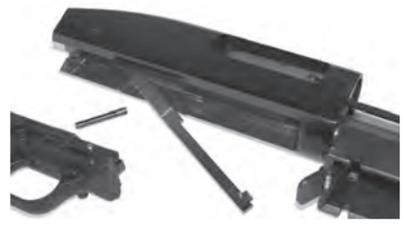
**7** Install trigger group by inserting front of trigger group up into the receiver and then swing rear of group up and into the receiver. DO NOT pull trigger during install.
