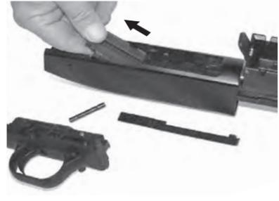
**8** Slide the forend forward and line up the follower assembly keeper with the opening on the top of the mag tube (A). Invert the firearm and allow the follower assembly keeper to fall free of the magazine tube (B). The action bar and forend assembly will now pull freely from the receiver and off the magazine tube.
