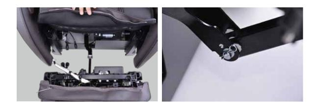
**Connect wires in footrest.** Connect footrest wire connectors and screw the caps tight. Then connect the air hose. **Caution:** Match the connectors and aline the white points before you connect them.
