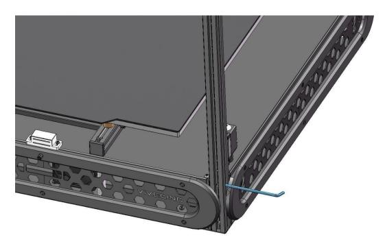
Repeat, tightening all four Z axis extrusions in place.
