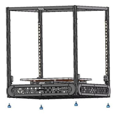
Put foam on print plate from the box. Pictured with top frame attached, but we suggest installing the gantry before the top frame to make it easier
