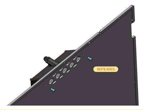
Install the screws first, holding the area with the VHB tape away from the panel, then press the VHB to the back panel. This will help in positioning the air filter.
