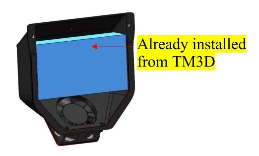
Attach air filter to the outside of the black real panel.
