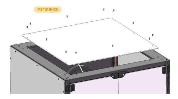
Remove the screw in below position.
