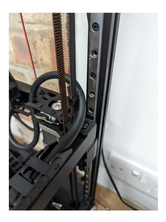
Slip the buckle onto belt over folded flap and tighten it with a M3 set screw.
