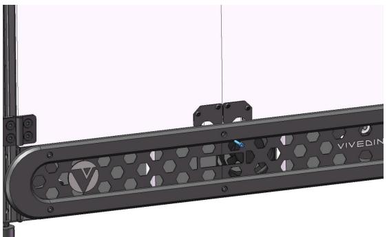
Connect the two ribbon cables according to the label behind screen, then mount the screen by screw.
