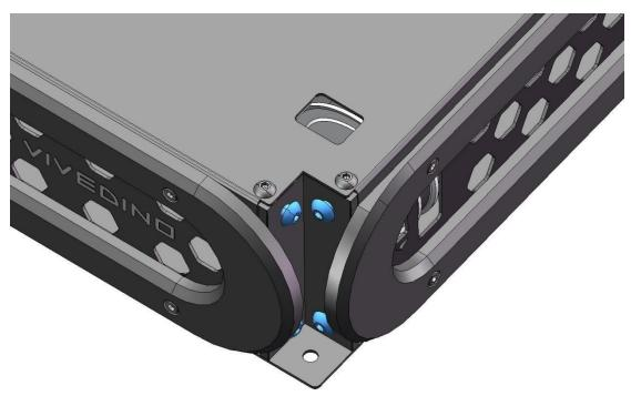
Install the Z axis extrusions making sure the ball is facing up. Be sure the extrusions are flush against the sheetmetal beneath the print bed. Tighten all of the screws (all 4 corners) until the extrusions are held in place (just past loose) then, fully tighten each screw.
