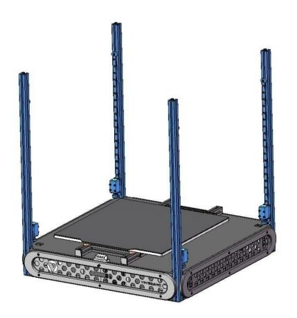
Mount the feet to the bottom of the printer. They are adjustable so you can level the machine in its final location.
