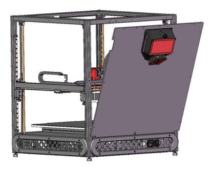
Pass cables through the bottom slot of Rear panel.
