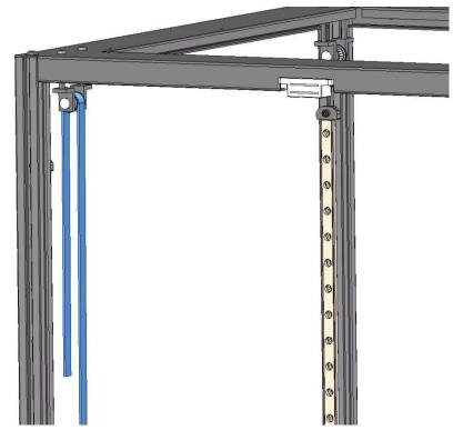
Slip a buckle onto the belt.
