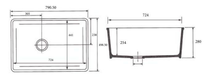
\* DUE TO THE MANUFACTURING PROCESS SINKS MAY HAVE SLIGHT VARIANCES IN SIZE. THESE DIMENSIONS SHOULD BE USED AS A GUIDE ONLY. WE STRONGLY RECOMMEND THE SINK BE ON SITE WHEN CABINETS OR BENCH TOPS ARE BEING PREPARED FOR THE SINK.
