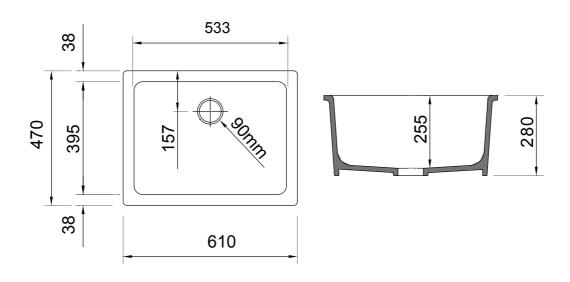
\* DUE TO THE MANUFACTURING PROCESS SINKS MAY HAVE SLIGHT VARIANCES IN SIZE. THESE DIMENSIONS SHOULD BE USED AS A GUIDE ONLY. WE STRONGLY RECOMMEND THE SINK BE ON SITE WHEN CABINETS OR BENCH TOPS ARE BEING PREPARED FOR THE SINK.
