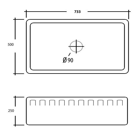
\* DUE TO THE MANUFACTURING PROCESS SINKS MAY HAVE SLIGHT VARIANCES IN SIZE. THESE DIMENSIONS SHOULD BE USED AS A GUIDE ONLY. WE STRONGLY RECOMMEND THE SINK BE ON SITE WHEN CABINETS OR BENCH TOPS ARE BEING PREPARED FOR THE SINK.
