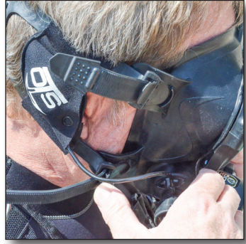
Figure 16: To Remove Mask, Use Thumbs to Grasp Bottom Buckle Tabs and Loosen
