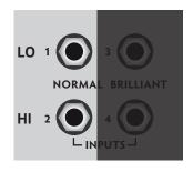
The NORMAL volume feeds a full range gain stage the delivers deep low end and a subtle top end sparkle. As you increase the volume, the tonal balance develops a fatter smoother character. This stage is ideal for dialing in a big dynamic punch that cleans up nicely when backing off on the guitar volume.
