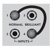
Jumping the inputs allows you to blend the NORMAL and BRILLIANT voicings. When jumping the inputs, use the short, shielded cable provided from the bottom NORMAL jack to the top BRILLIANT jack or vice versa. In either case plug your guitar into the remaining bottom jack (Input 2 or 4) for best tone and sustain.
