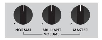
The NORMAL and BRILLIANT volume controls set the input stage gain amount as you rotate the knob clockwise. Each stage features dual input jack pairs. In each pair, the bottom jack is 3dB hotter that the top jack.
