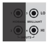
The BRILLIANT volume feeds a somewhat hotter gain stage with a rolled off low end and a pronounced midrange emphasis. As the gain is increased, the tonal balance is shifts from upper mid emphasis to a lower mid emphasis with a noticeable onset of preamp distortion. This will produce a thick meaty tone. The forward top end voicing of this stage allows you to turn down the tone control on your guitar for a sweet sustaining "Woman Tone" vibe.
