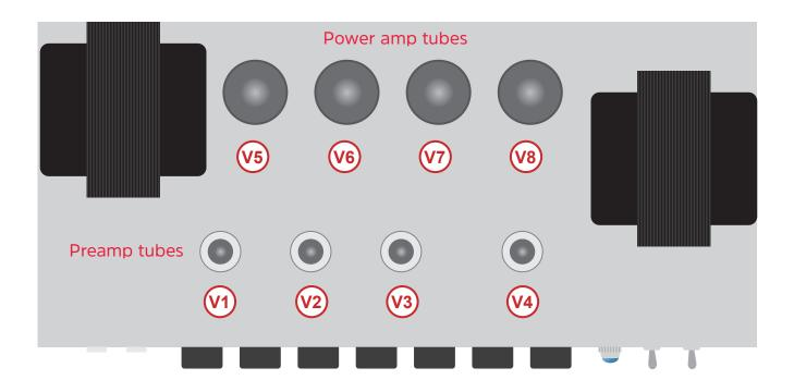
Tube locations are from right to left looking at the back of the amp. Tube types are factory selected for superior performance, consistent tone quality and reliability. While substituting other brands may not cause damage to the amplifier this may affect amplifier performance in unpredictable ways. For best performance, replace only with factory recommended tubes. Warning! Substituting other tube types is not recommended.
