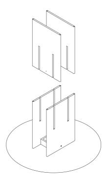
Next, fit the other base-panels (D) into the frame of the already fixed panels (C).
