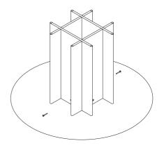
Last, gently tighten the bolts (A) with the included hex key (B) when all the panels are in the right place. Finally, turn the table and enjoy.
