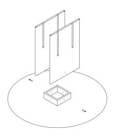
First, place the tabletop on a protective surface or carpet with the bottom facing upwards. Then fix the base panels (C) to opposite sides of the socket on the table top (E). Gently tighten the bolts (A) with the supplied hex key (B)
