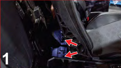
1 SLIDE SEAT FORWARD AND REMOVE BOTH BOLTS FROM FLOOR
