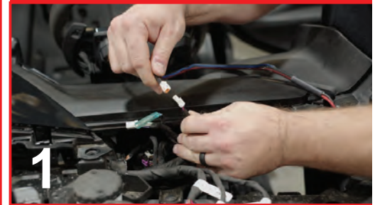
1 PLUG IN THE WHITE HARNESS PLUG INTO THE SMALLER OEM PLUG
