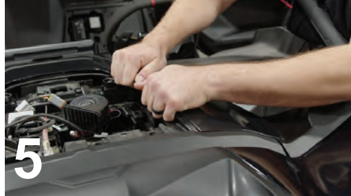
5 REMOVE THE DASH PANEL
