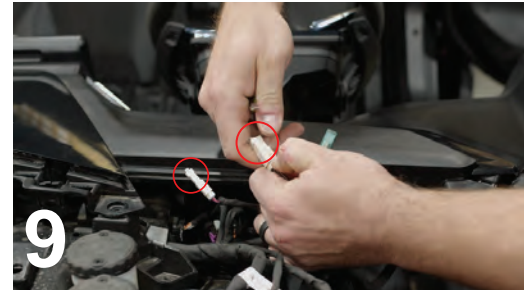
9 REMOVE THE OEM CAPS ON BOTH PLUGS
