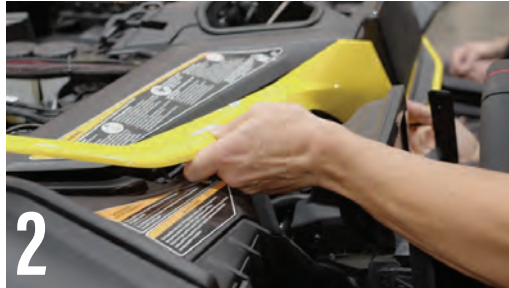
2 REMOVE THE THREE YELLOW PLASTIC TRIMP PANELS (DRIVER SIDE, CENTER PIECE, PASSENGER SIDE)
