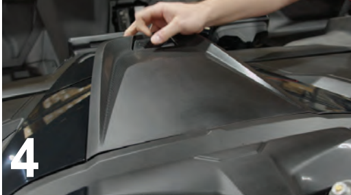
4 REMOVE THE HOOD PIECE
