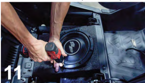
11 USE THE SCREWS INCLUDED WITH SUBWOOFER TO SECURELY FASTEN THE SUBWOOFER TO THE ENCLOSURE
