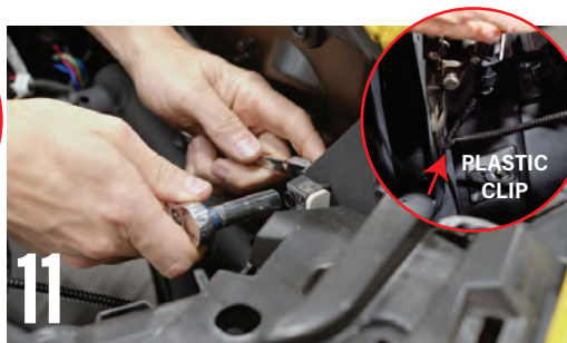
11 REMOVE THE 10MM SCREW HOLDING ON THE (?) SENSOR
