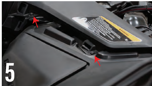
5 REMOVE THE TWO SCREWS ABOVE GLOVE BOX ON PASSENGER SIDE
