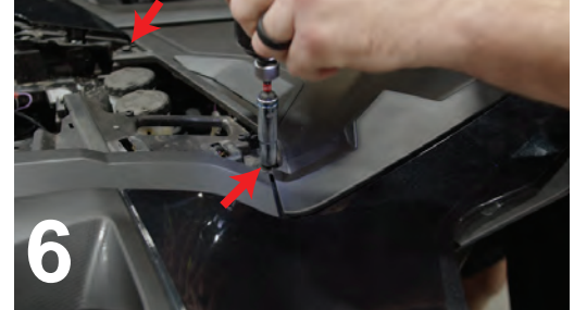
6 REMOVE BOTH 10MM BOLTS
