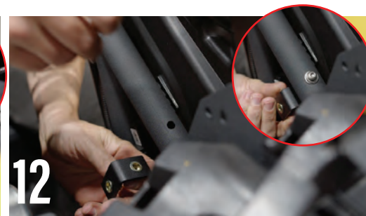
12 PLACE THE L-BRACKET ONTO THE DRIVER SIDE FRAME AND SECURE IT USING THE INCLUDED HARDWARE
