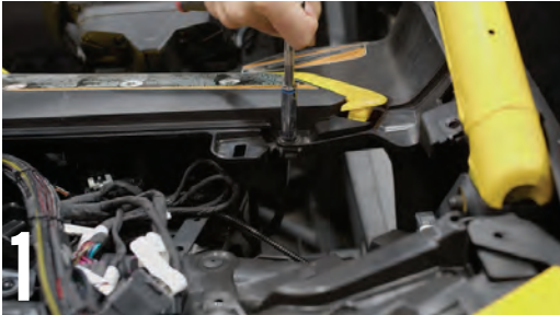
1 REMOVE 10MM SCREW IN DASH
