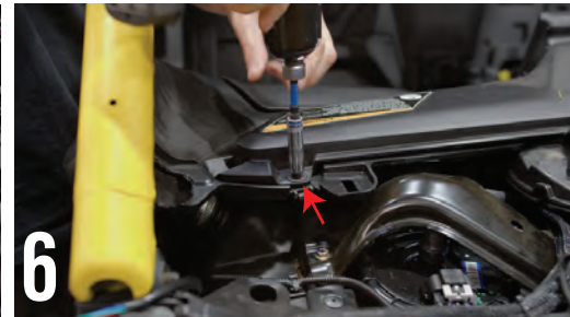
6 REMOVE THE LAST SCREW ON DASH JUST ABOVE GLOVE BOX
