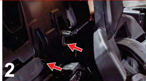
2 REMOVE THE BOLTS FOR THE HARNESS LOCK MECHANISM
