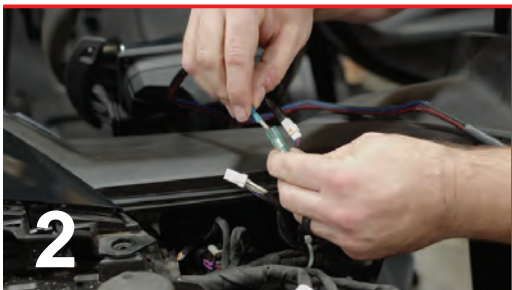
2 CONNECT THE REMOTE (BLUE) WIRE
