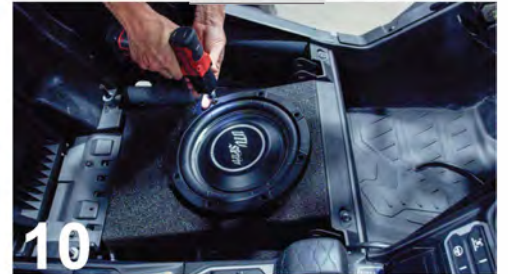
10 ALIGN SUBWOOFER ON ENCLOSURE AND PRE-DRILL THE HOLES
