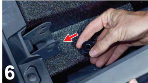
6 USE THE BLACK SPACER FROM STEP 1 AND SLIDE UNDER THE SEAT MOUNT BRACKET
