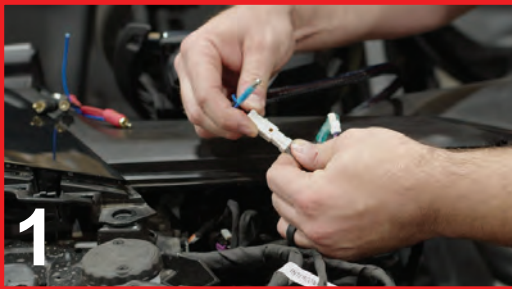
1 PLUG IN THE WHITE HARNESS PLUG INTO THE LARGER OEM PLUG
