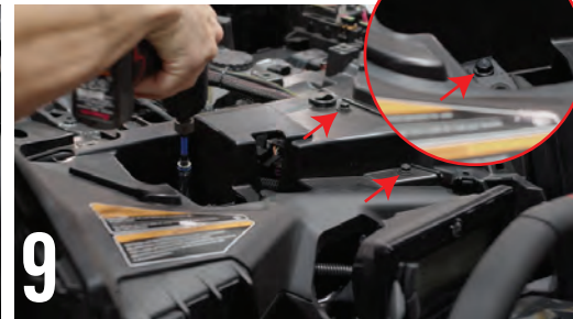
9 REMOVE THE THREE SCREWS SHOWN HERE BEHIND THE STEERING WHEEL
