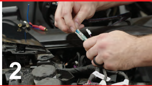
2 CONNECT THE REMOTE (BLUE) WIRE
