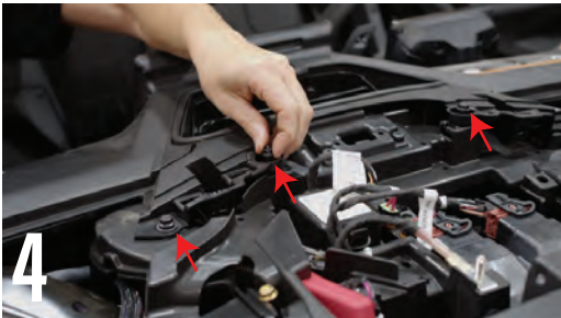
4 REMOVE 3 SCREWS LOCATED UNDER DASH PANEL
