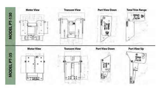
Note: The inside dimension of the motor mounting area of the PT-35 is 11". Before ordering, please make sure that the maximum width of the clamp mounting feet and/or mounting bolts of the motor that must fit into this area does not exceed the 11" limit. Refer to the transom view drawings. Mounting bolts are not included with the PT-35.
