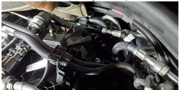
9. Route the sensor electrical harness to the brake booster/master cylinder compartment on the driverside.
