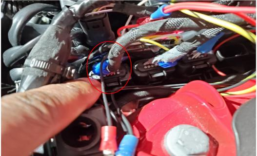
**NOTE:** The Zeitronix module mount location is up to the user. We placed ours in the Master Cylinder compartment on the driverside. Doing this allows you to only need to run one wire through the firewall. And that would be for the ZT gauge. In that event please see below for firewall routing.
