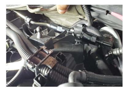
8. Reconnect the factory low pressure fuel line to the sensor and low-pressure hard line. Re-install the vacuum canister. Re-install the grayish/white plastic clip to the fuel line closest to the strut tower. And use the supplied Black clip for securing the sensor side quick disconnect.
