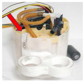
11. Drill two 4mm holes in the OEM assembly using the locator holes on the pump bracket indicated by the two red arrows. Clean out leftover debris in the bucket if any.
