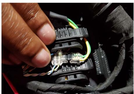
25. Go back to the truck, connect the pump harness via the plug connector to the Relay. And connect the main power and ground leads of the relay to the battery.
