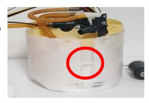
10. Install the Twisted Tuning pump pump bracket onto the OEM pump assembly using the bracket mount positioning slot of the OEM bucket indicated by the red arrow in the image below. Make sure its seated and level.
