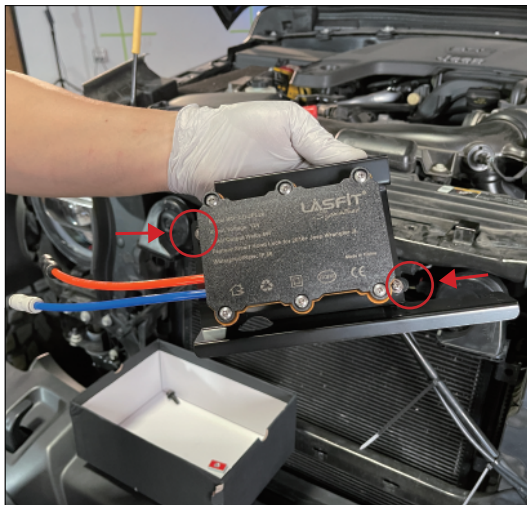
4.1 Fix controller box on the mounting bracket.
