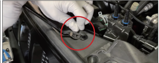
1.2 Remove the six plastic clips with a trim removal tool.
