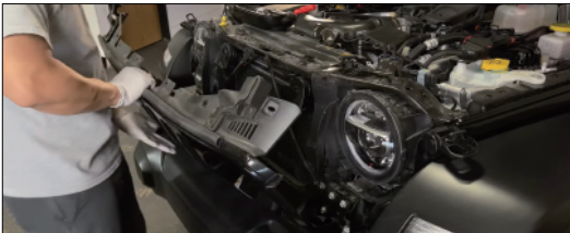
1.3 Remove the front grill by slightly pulling the top up.
