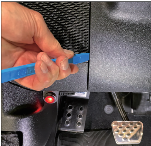
4.2 Remove the panel under the steering wheel using the trim removal tool.
