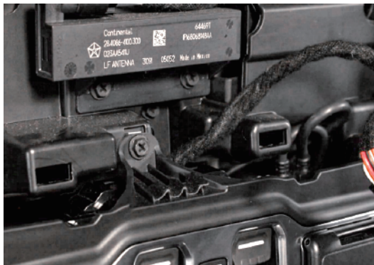
6.1 Reinstall the screw back to the dash.
