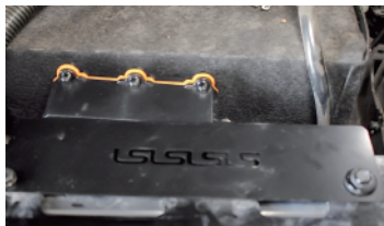
1.3 Mount the bracket(s) with the power distribution.
