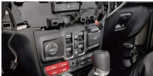
5.8 Put the panel back on with newly-installed switches.
