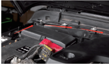
2.1 Route and ziptie the wires all the way over to the driver's side.
