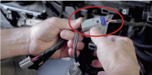
5.2 Connect the factory cigarette lighter harness (with the blue tab) with our supplied harnesses.
