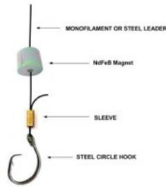
Detail of a rare earth magnet secured on a longline gangion.
