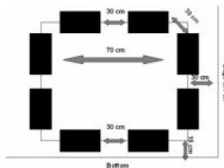
*Detail of an opening in the fence. Permanent magnets are secured around the perimeter of the opening to selectively exclude elasmobranchs.*
