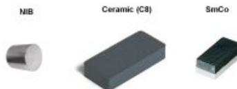
The fields generated by these permanent magnets (shown above) decreases at the inverse cube of the distance from the magnet to sharks and rays. Therefore, at distances of a few meters from the magnet, the field exerted is less than the Earth's magnetic field. Animals which lack that Ampullae of Lorenzini organ do not display aversive behavior in close proximity to the magnetic field, making this technology selective
