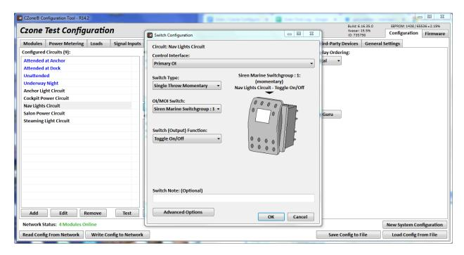
That will allow the circuit to be controlled by both "All Display Interfaces" and "Siren Marine Switchgroup: 1." Siren Marine Switchgroup is controlled by the Siren Marine Unit and the Nav lights Circuit is now mapped to switch 1 on that interface.
