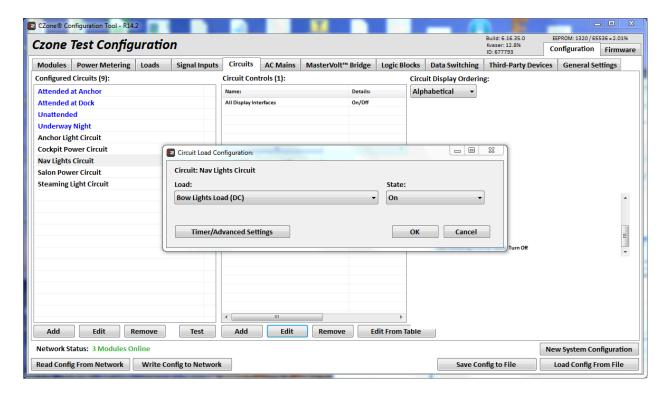
Click "OK" to save it, and then repeat this procedure to add any additional loads you want controlled by this circuit. The screenshot below demonstrates a newly added circuit called "Nav Lights Circuit" which controls both the bow lights and the stern light.
