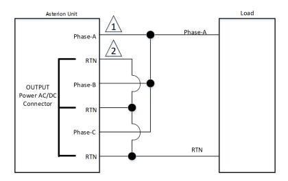
Figure 3-10. Output Connection to 1-Phase Load
