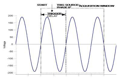
Figure 6-6. Pre-Trigger (Negative Delay
