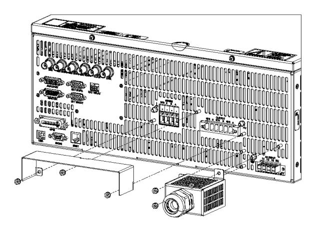
Figure 3-2. Rear Panel Protective Cover Installation
