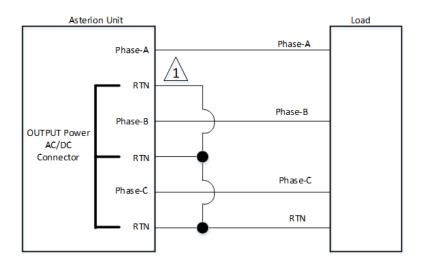
Figure 3-9. Output Connection to 3-Phase Load
