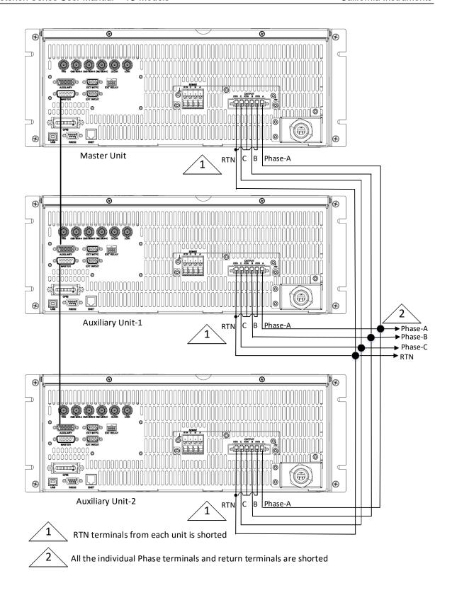
Figure 3-22. Connections for 3-Phase Parallel Group
