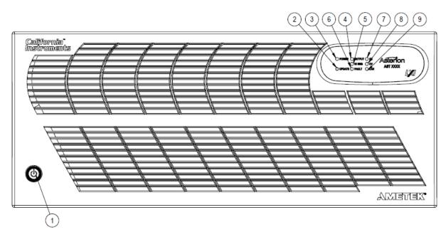
Figure 4-2. Front Panel, ATE Models
