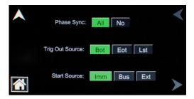
Figure 4-23. SETTINGS Screen, TRIGGER Sub-Menu
