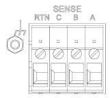
Figure 3-11. Remote Sense Connector and Functional-Ground
