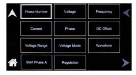
Figure 4-16. OUTPUT PROGRAM Screen Top-Level Menu
