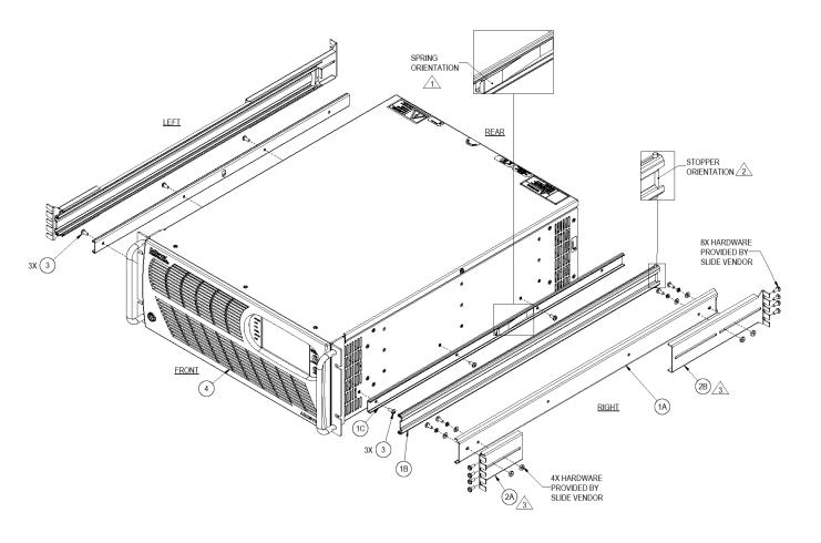
Figure 3-1. Rackmounting Installation
