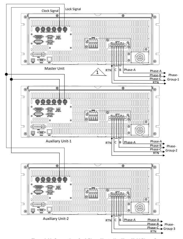
Figure 3-23. Connections for 3-Phase Master/Auxiliary Multi-Phase Group
