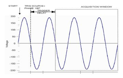
Figure 6-5. Post-Trigger (Positive Delay)
