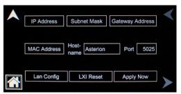
Figure 4-45. CONTROL INTERFACE, LAN CONFIGURE Sub-Menu
