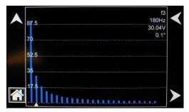
Figure 6-3. FFT data in Bar Graph Format
