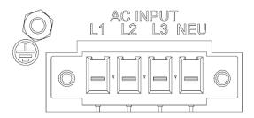
Figure 3-7. AC Input Connector and Safety-Ground Stud, for 4-Wire (with Neutral) plus Ground Input
