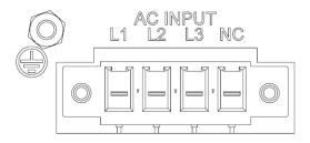
Figure 3-6. AC Input Connector and Safety-Ground Stud for 3-wire plus Ground Input
