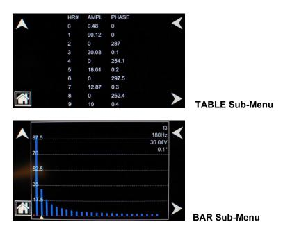
Figure 5-1. HARMONICS Screen, Waveform Information
