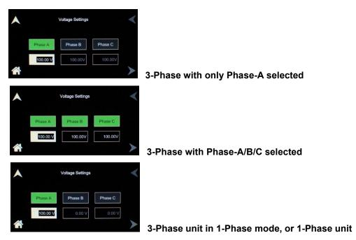
Figure 4-10. Highlighted Voltage Selection-Field with Value Window
