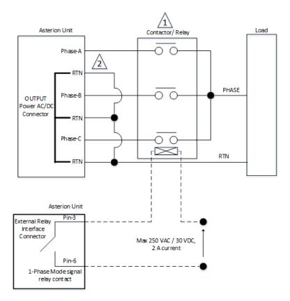
Figure 3-14. External Relay Interface for 1-Phase Relay Control
