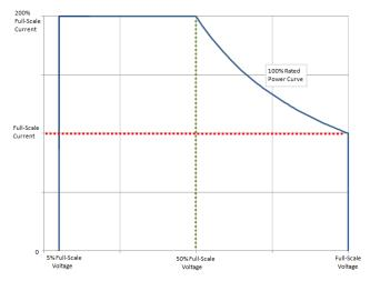
Figure 4-3. iX2<sup>™</sup> Constant-Power Output Characteristic
