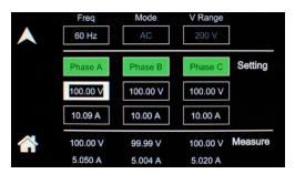
Figure 4-5. DASHBOARD Screen Menu with Voltage Selection-Field Active
