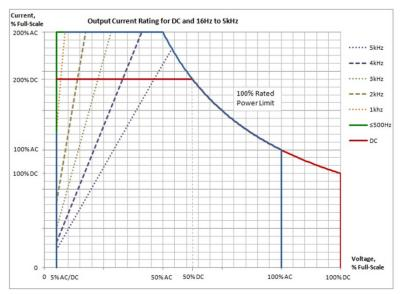
Figure 2-1. iX2<sup>™</sup> Constant-Power: Output Current Versus Voltage, AST 4503 3-Wire Input, AST 6003
