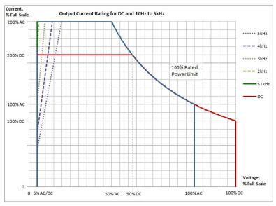
Figure 2-2. iX2<sup>™</sup> Constant-Power: Output Current Versus Voltage, AST 4503 4-Wire Input
