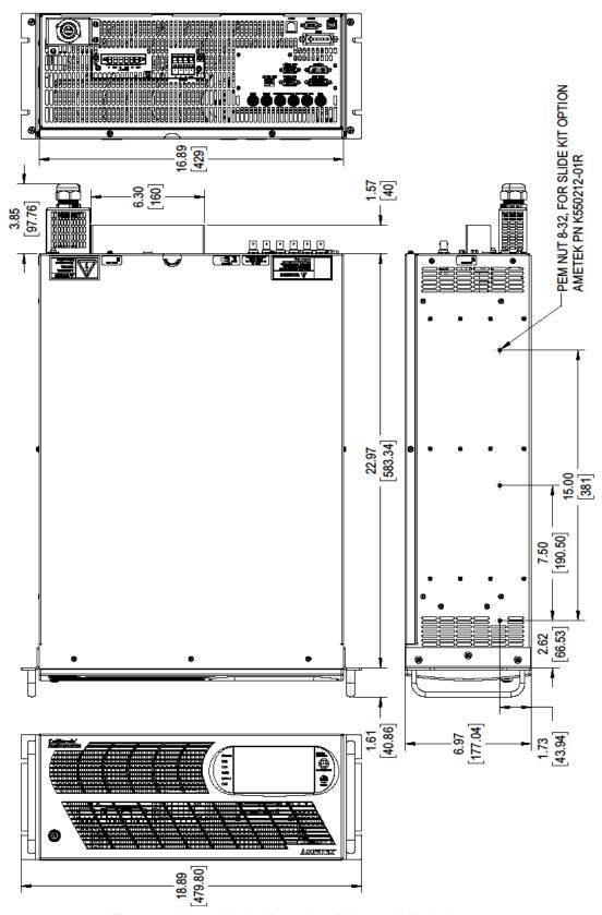
Figure 3-3. Installation Drawing, Enhanced Models
