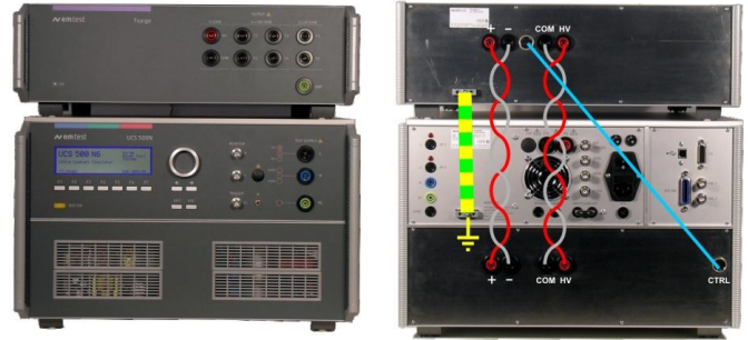
Test Setup UCS500N7 and TSurge7
