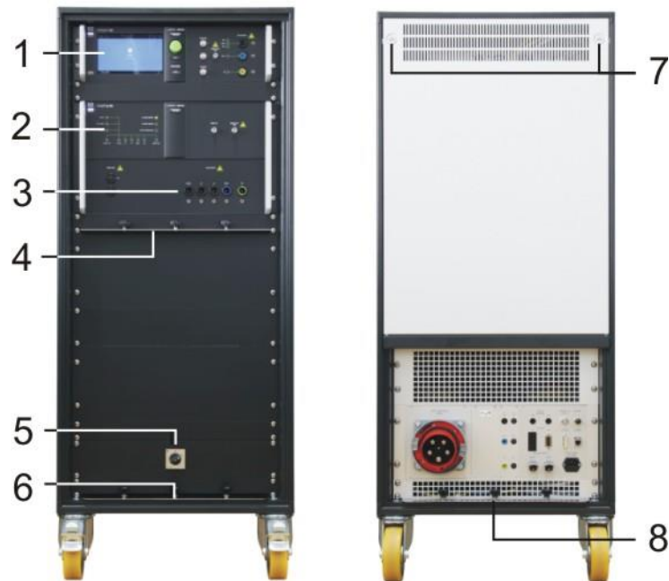
Figure 5.3: Test system with compact NX5, coupling NX5 (model for EUT 3 x 480V /125 A)
