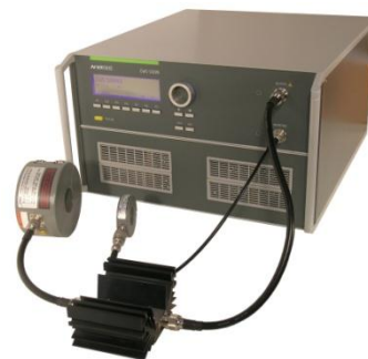
Figure 2.3a / 2.3b : Typical test setup with required parts for BCI application with CWS 500N2
