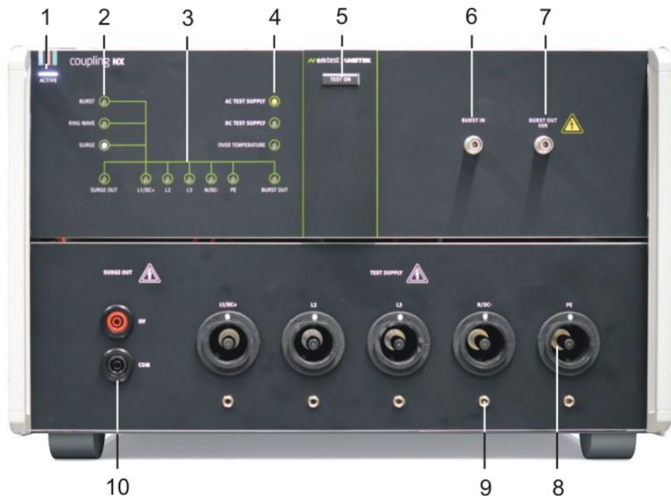
Figure 5.3: Test system with compact NX5, coupling NX5 (model for EUT 3 x 480V /200 A
