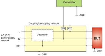
IEC 61000-4-18 Ed1 figure 11a Setup implemented with the ground reference plane IEC 61000-4-18 Ed1 figure 11b Setup implemented with dedicated earth connection
