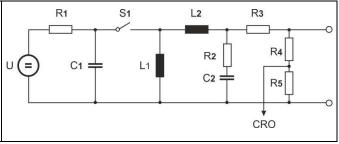
Block diagram Damped oscillatory Wave Generator
