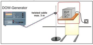
At 1 MHz test, the cables (max. 3 m) must be twisted
