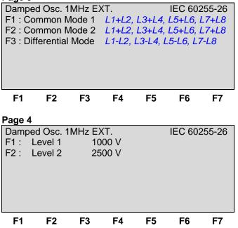
The standard levels for common and differential mode can be changed in the setup menu.
