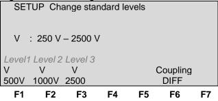
**F1, F2, F3** For each coupling (Differential mode and Common mode) a separate level can be settled. The display shows the actual working mode.
