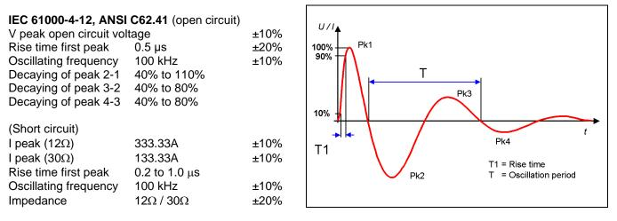
Remark: The output impedance is calculated result of the ratio of the first peak open circuit voltage and the first peak short current, measured with a 4000V pulse.
