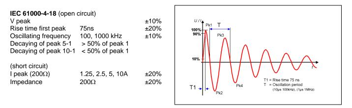
Remark: The output impedance is calculated result of the ratio of the first peak open circuit voltage and the first peak short current, measured with a 2500V pulse.
