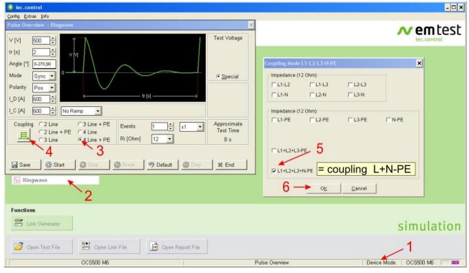
Figure 11.1: Coupling L+N-PE with software IEC.control
