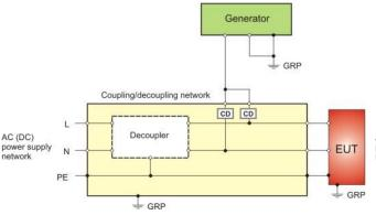
IEC 61000-4-18 Ed1 figure 7a Setup implemented with the ground reference plane
