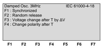
After selection the last used test parameters will be indicated on the display.
