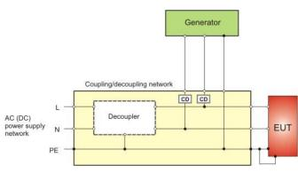
Test setup for Line to Line test
