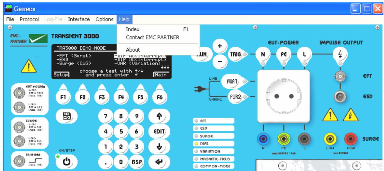
The GENECS windows is identical to the TRA3000 F-S-D-V-C front plate. Online the TRA3000 F-S-D-V-C can be remote controlled by pressing the buttons with the mouse cursor as on the real front plate.
