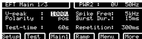
The screenshot shows the test parameters menu for 'EFT Main 1/3'. It displays various parameters: 'U-peak : 1000V', 'Polarity : pos', 'Test-time : 60s', 'Spike Freq: 5kHz', 'Burst Dur.: 15ms', and 'Repetition: 300ms'. At the top right, it shows 'PRK2 : 00 50Hz'. At the bottom, there are navigation buttons: 'Setup', 'Test', 'Main1', 'Ramp', 'Menu', and 'More'.
