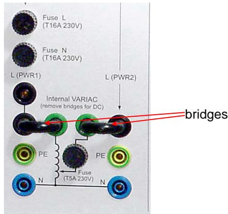
Both bridges must be placed as shown in the picture . EUT Power 1 must be connected to the 230 V public power supply.
