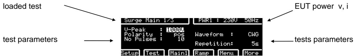
When the EDIT button has been pressed the dialogue line indicates the possible range like v, time, etc.
