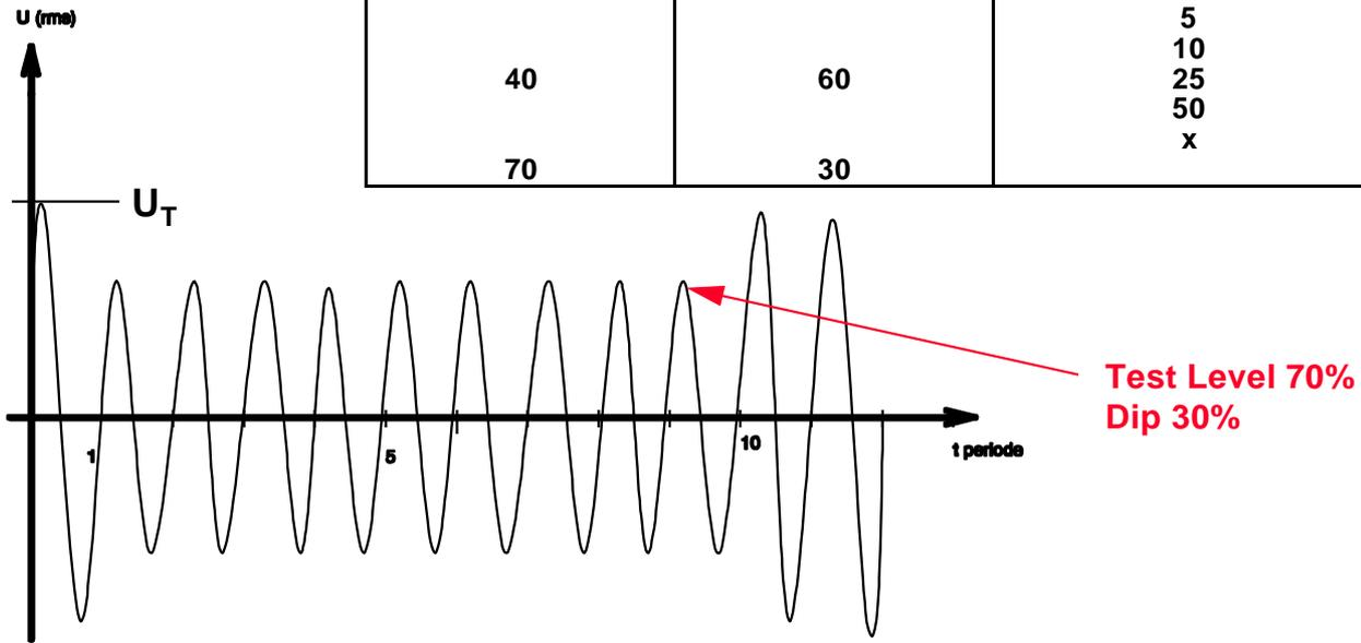
In addition to the data showed in the figure, such as test levels, duration of the interruption, transition time, etc., the inrush current must be tested. Electronic equipment very often contain inrush current limitation circuits. These inrush limiting circuits are often bypassed during interrupts at the turn on part. Consequences are defective power switching modules, or the equipment can not be turned on after the test because the software has not made a restart etc.
