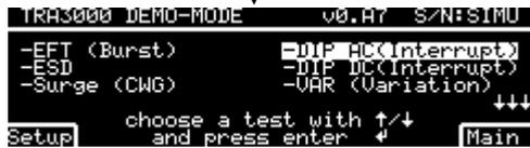
The screenshot shows the main menu of the TRA3000. At the top, it displays 'TRA3000 DEMO-MODE v0.47 S/N:SIMU'. Below this, there are two columns of selectable tests: '-EFT (Burst)', '-ESD', and '-Surge (CWG)' on the left; and '-DIP AC(Interrupt)', '-DIP DC(Interrupt)', and '-VAR (Variation)' on the right. A prompt at the bottom says 'choose a test with ↑/↓ and press enter ↵'. Navigation buttons 'Setup' and 'Main' are visible at the bottom corners.
