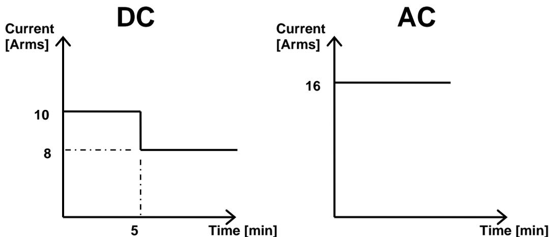
**A temperature sensor protects the high voltage switch in case of d.c. supply.**
