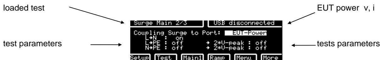
When the 2 x V-peak are selected "on" the voltage of the L→N voltage will be doubled as specified in the standard for common and differential tests.
