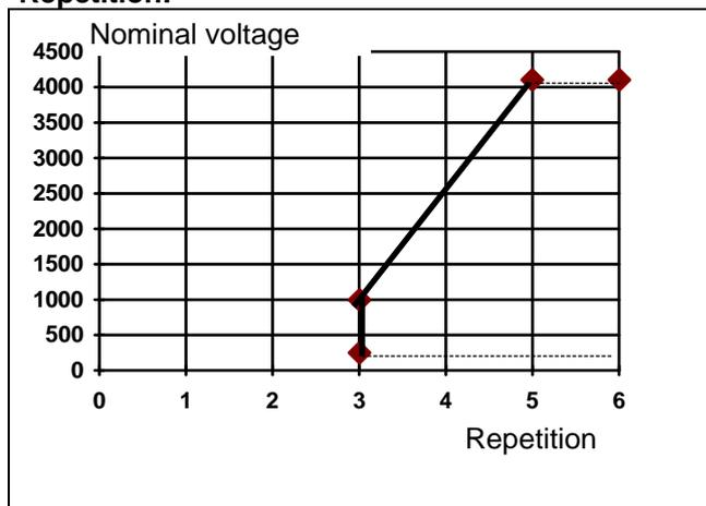
Repetition is defined as the time between two successive impulses. For each discharge the capacitor in the TRA3000 F-S-D-V-C must be charged. The stored energy is a function of the charging voltage, therefore the repetition rate is a function of the voltage.
