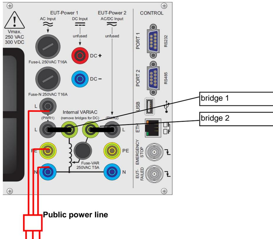
The Bridge 1 connects the internal variac with the public power supply on the primary side.
