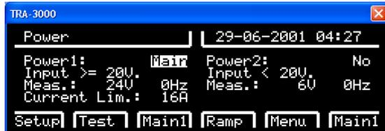
(voltage PWR1 and PWR2 must be selected on external power supplies)
