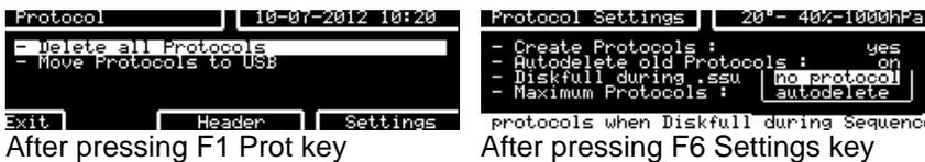
This function relates to sequences stored and run from the TRA3000 F-S-D-V internal memory. It is an extension to the “Autodelete old protocols” function.
