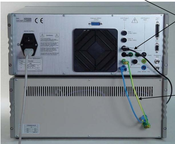
Cable for the synchronisation. Please use the 1 m black cable delivered with the CDN2000 to synchronize the TRA3000 F-S-D-V-C with the desired phase of the CDN2000.
