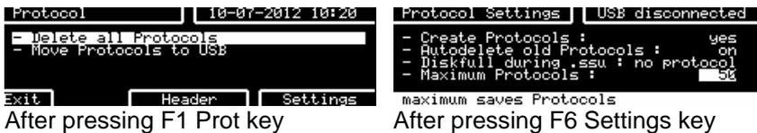
This function defines the maximum number of protocols that can be saved in TRA3000 F-S-D-V internal memory. If this value is exceeded, the oldest protocols will automatically be deleted. First-in-first-out. Default value is 50.
