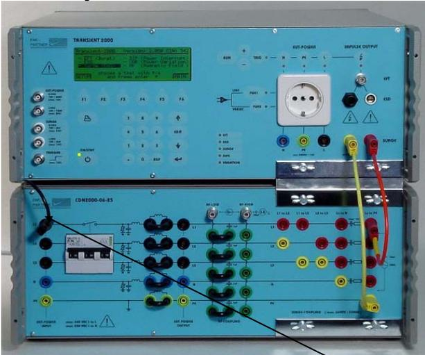
Different possibilities exist to synchronize the TRA-generator with a three phase coupling filter.
