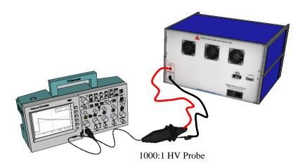
Figure 9. Energy Measurement with an External Acquisition System
