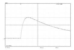
Figure 6. Vpeak = 3.88kV with 25mH inductor
