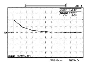
Figure 10. Y1-Y2 Waveform using a Defib-5P Pass/Fail Reference
