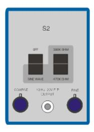
Figure 13. Sine Wave Generator option
