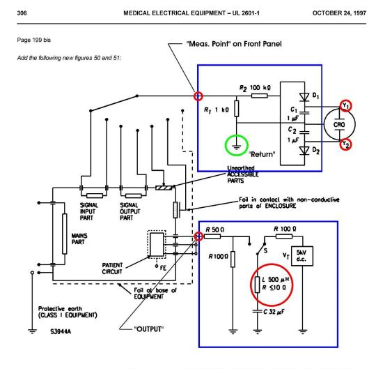
Figure 50 – Application of test voltage to bridged PATIENT CONNECTIONS for DEFIBRILLATION-PROOF APPLIED PARTS (see subclause 17 \*h))
