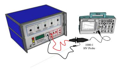
Figure 4. Checkout Pulse Setup
