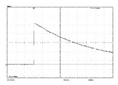
Figure 5. Vpeak = 4.72kV with 500uH inductor
