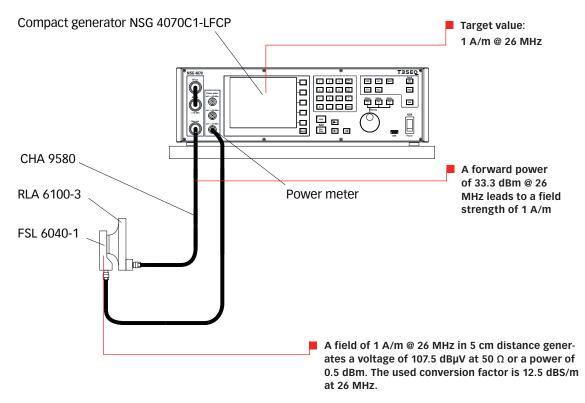
Figure 1: Set up example for test level setting for the whole frequency range
