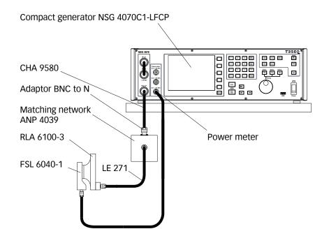
Figure 2: Set up example for test level setting for the frequency 13.56 MHz with ANP 4039
