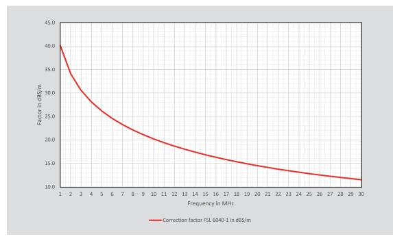
Figure 9: FSL 6040-1 Field Sensor Loop typical correction factor 1 MHz to 30 MHz
