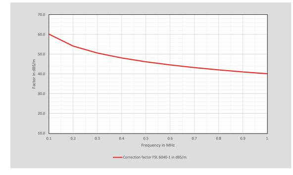
Figure 8: FSL 6040-1 Field Sensor Loop typical correction factor 100 kHz to 1 MHz
