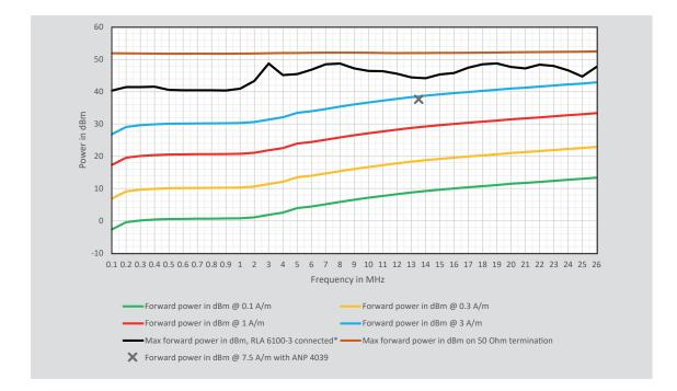
\* The display of the forward power via a 50 Ohm power meter at the directional coupler is distorted by the strong mismatch. It can therefore only be used to a limited extent. Likewise, the output power of an amplifier is dependent on the connected load.
