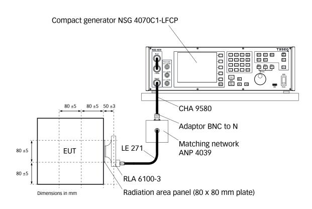
Figure 4: Set up example for testing the frequency 13.56 MHz with ANP 4039
