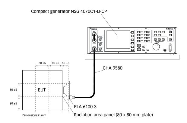
Figure 3: Set up example for testing
