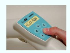
As showed above the "RUN" button must be pressed until the message is shown "power down".
