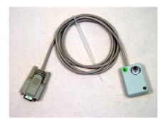
The serial port uses just the data lines TxD and RxD for information transfer (9600Baud, 8 N 1).
