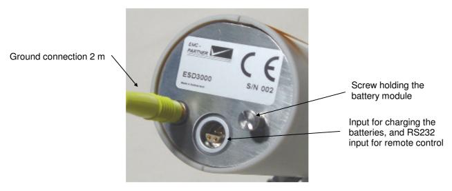
The control of the ESD3000 is carried out by a microprocessor. The microprocessor controls the EMC tests, stores the inputs of the numeric input terminal, updates the display, checks whether the inputs of the operators are allowed values or not. The operator communicates with the ESD3000 via the input terminal and the display.
