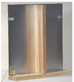
Vertical coupling plate. Mechanical dimension: 0.5 x 0.5 m Application indirect ESD discharge with contact tip.
