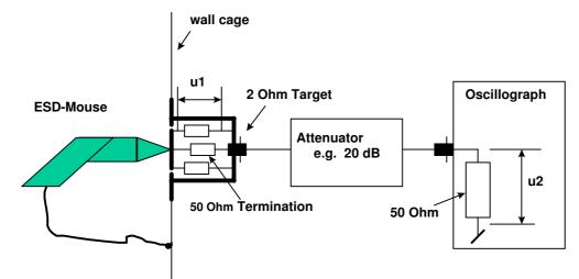
The ESD-current produces on 2 Ohm Shunt a voltage trop u1. The 2 Ohm target is terminated with 50 Ohm to avoid reflection. With the 20 dB attenuator the 60V trop on the 2 Ohm will be reduced to the allowed input voltage of the oscilloscope. The memory oscilloscope must have a minimum bandwidth of 1 GHz. For all four levels (2,4,6,8 kV) the current wave-form must be within the tolerances as specified in the IEC standard 61000-4-2.
