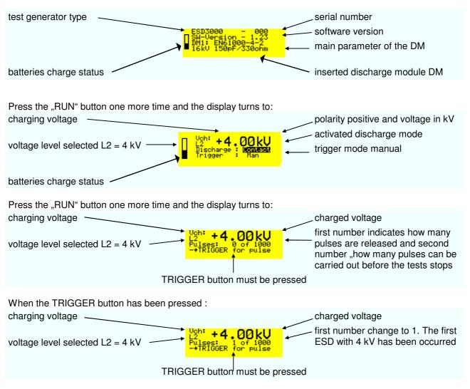
Press the "RUN" button and the ESD3000 return to the main setting mode.
