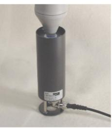
20 G divider for high voltage measurement on the ESD3000 up to 25 kV. Ratio is determined by 1 M Ohm input of the oscilloscope. Ration approximate 20'000
