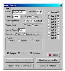
Click 'Load Setup' to enter the parameter input menu (picture left). Parameters can be changed and saved in one of 9 memory locations on the computer hard disk. These setup files can be transferred to the ESD3000 using the download module.
