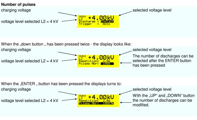
**Remark:** up to 1000 discharges steps are 1, over 1000 steps change to 1000. Holding the "UP" or "DOWN" button pressed, the steps changes from 1 to 10 or from slow to fast.
