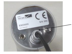
Connect the special Lemo connector to the ESD3000 on the bottom side. The power supply cord must be connected to a public outlet with voltage 110 V up to 240 V 50/60 Hz
