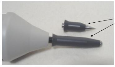
Pull out the finger and insert the tip
