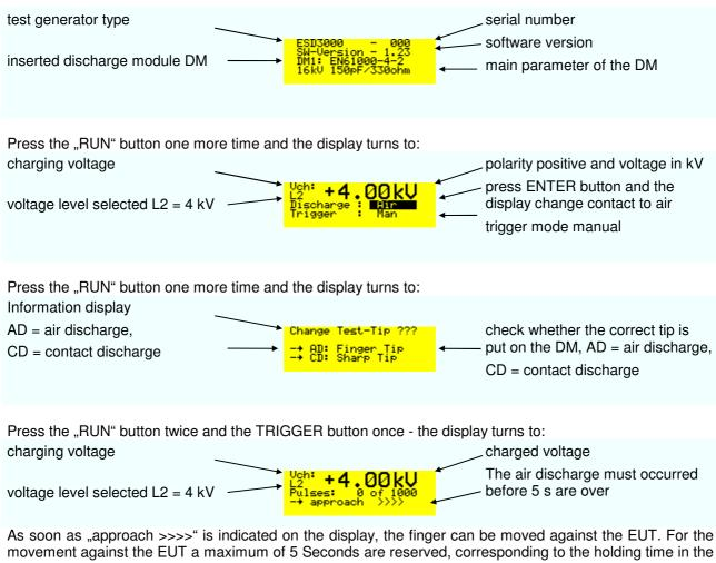
As soon as "approach >>>> is indicated on the display, the finger can be moved against the EUT. For the movement against the EUT a maximum of 5 Seconds are reserved, corresponding to the holding time in the IEC standard. For ISO 10605 test on insulated equipment press the Trigger button a second time when the 15 mm position is reached. This will avoid second air discharges.
