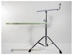
Height adjustable from 0.4 m up to 1.75 m Application: long term tests in contact and air discharge mode
