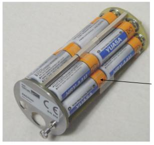
replace the batteries by pull it out piece by piece
