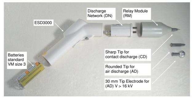
ESD3000 Contact Discharge (CD) up to 30 kV) with Relay Module (RM), Discharge Network (DN)
