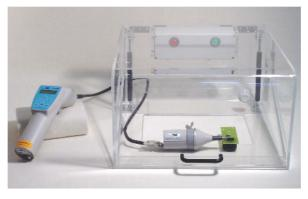
Testing of EUTs that could spontaneously explode or rapidly change state, such as airbags or munitions fuses
