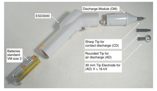
3.2.2 ESD3000 Contact Discharge (CD) up to max. 30kV with (RM and (DM )
