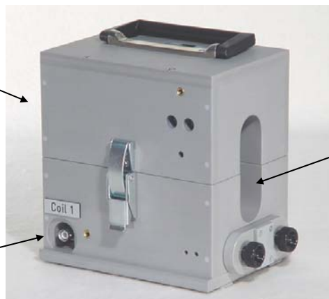
High voltage BNC input to connect coupler with generator Coil 2 level calibrated with the generator. Coil 1 only for evaluation process e.g. higher voltages
