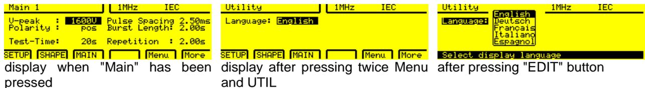
Chose the desired language (e.g. Spanish) with the arrows and quit with the ENTER button and press soft key F2 "TEST". The display "TEST" has now changed to
