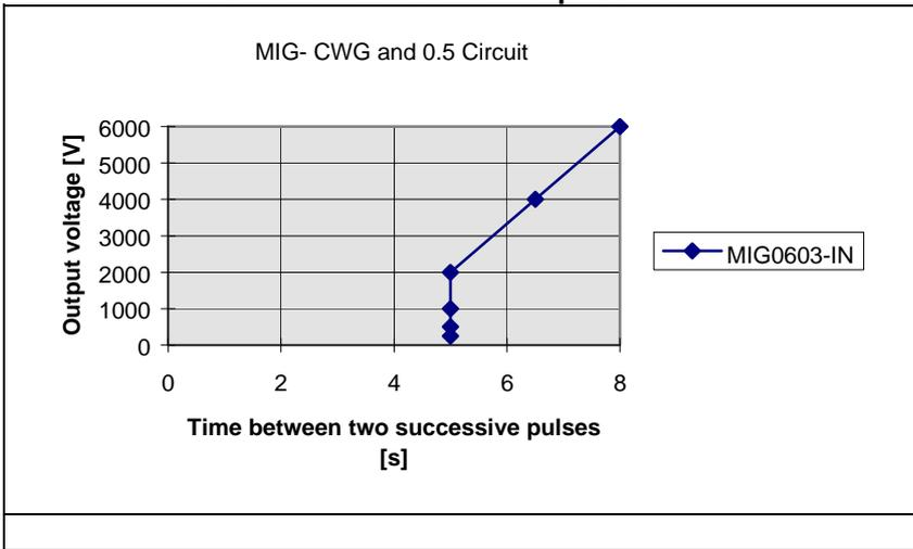
Repetition is defined as the time between two successive impulses. For each discharge the capacitor in the MIG0603-Oxx must be charged. The stored energy is a function of the charging voltage, therefore the repetition rate is a function of the voltage.
