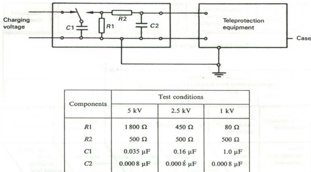
FIG. 5. — Circuit for impulse generator.
