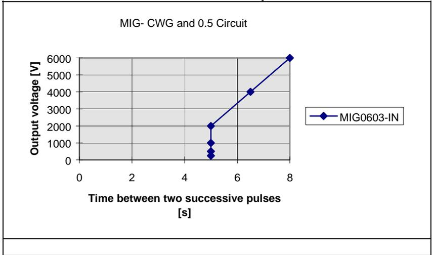
Repetition is defined as the time between two successive impulses. For each discharge the capacitor in the MIG0603-Oxx must be charged. The stored energy is a function of the charging voltage, therefore the repetition rate is a function of the voltage.
