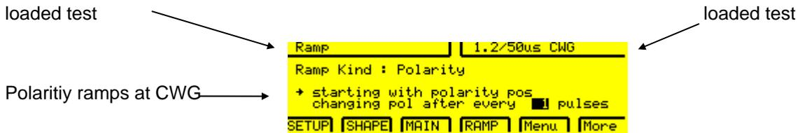
The polarity change „change after“ number of pulses. Start is always with the polarity selected in „Main Menu“.
