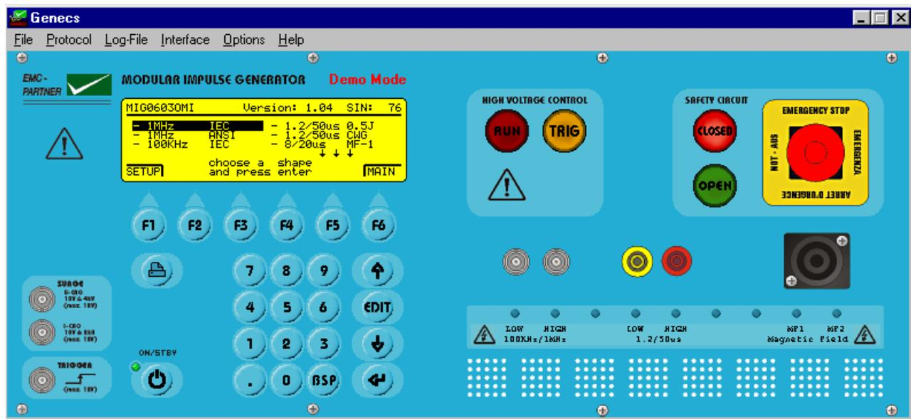
The GENECS windows is equal the MIG tester front plate. Online the MIG tester can be remote controlled by pressing the buttons with the mouse cursor as on the real front plate.
