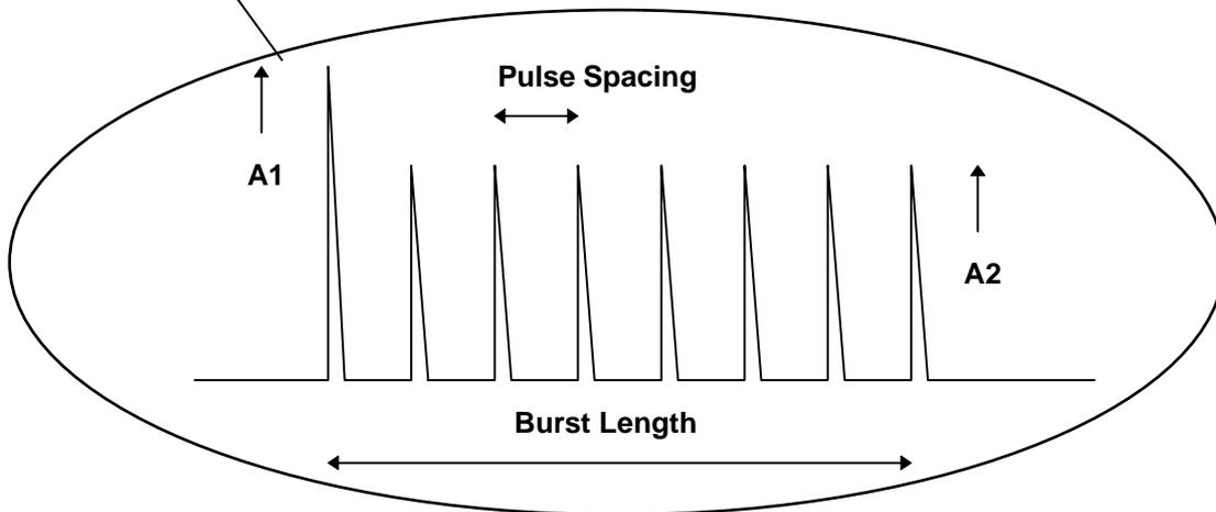
With pulse spacing the repetition frequency of the 1MHz or 100 kHz can be selected  $1/\text{periode} = \text{frequency}$ . e.g. 400 Hz = 2.5 ms pulse spacing
