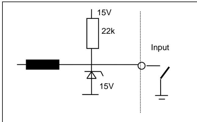
The trigger value at the output is approximately 3V
