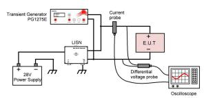
The automation software together with the voltage probe, the current probe and the oscilloscope can monitor the energy content of the spike and of the surge.
