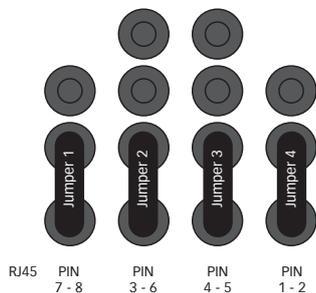
Figure 11: Jumper settings for 1000BaseT, 100BaseT4
