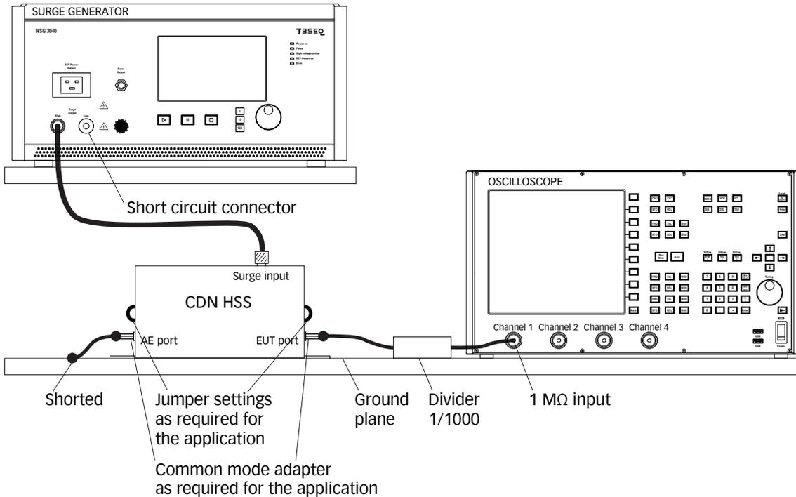
**Figure 12: Example of a setup for verifying the pulse parameters with measuring the open-circuit voltage**
