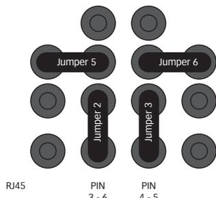
Figure 8: Jumper settings for ISDN basic rate access, S0
