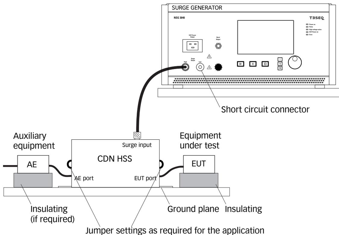
**Figure 5: Setup example with CDN HSS-2**
