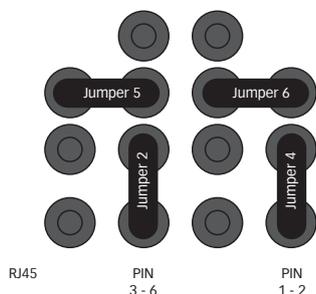
Figure 10: Jumper settings for 10BaseT, 100BaseT
