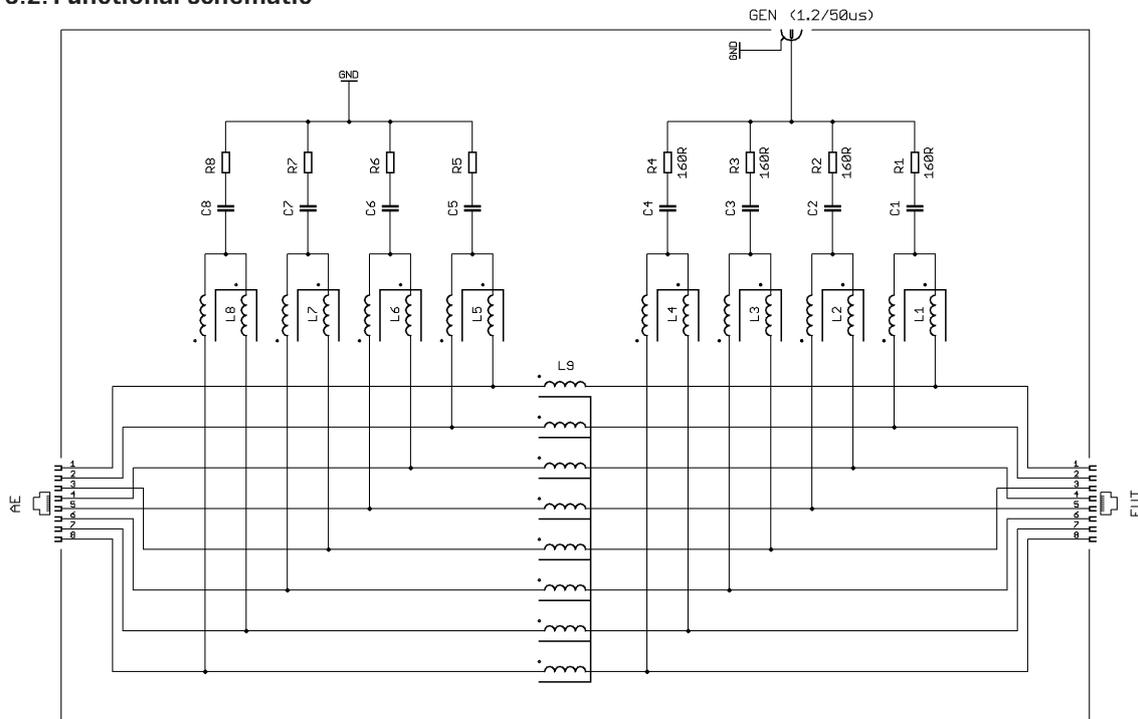
Figure 1: Functional schematic of the CDN HSS-2
