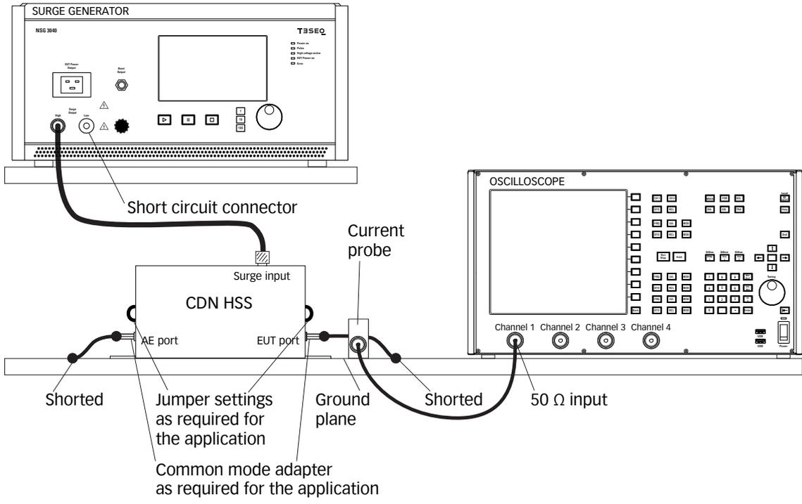
Figure 14: Example of a setup for verifying the pulse parameters with measuring the short-circuit current
