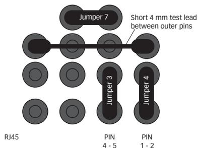
Figure 9: Jumper settings for ISDN primary rate access
