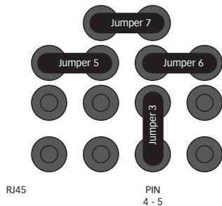
Figure 7: Jumper settings for testing on pin 4 and 5
