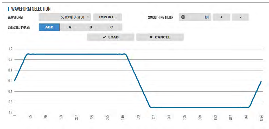
Figure 6-7: Same Waveform with maximum smoothing Filter Applied
