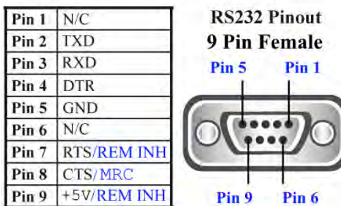
Figure 5-25: Remote Inhibit Pins on DB9 for AFX-2L and AFX-4L Versions
