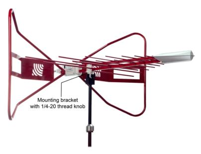
Model 3142E shown in horizontal polarization
