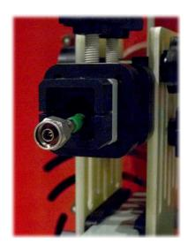
2. Attach the cable to the Type N connector at the end of the stinger.
