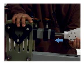
4. When you reach the back of the balun box, align it with the boom receptacle, and then slide the smaller portion of the balun box into the boom. This will prevent rotation of the antenna unless the boom is being polarized.
