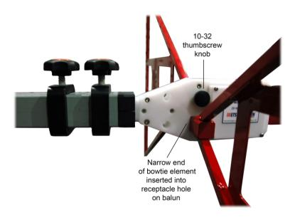
2. Slide the narrow end of one of the bowtie elements into the receptacle hole on the antenna balun, and then align the bowtie with the receptacle on the balun.
