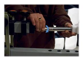
3. Slide the cable and stinger into the clamp on the boom, carefully guiding the cable out the other end.
