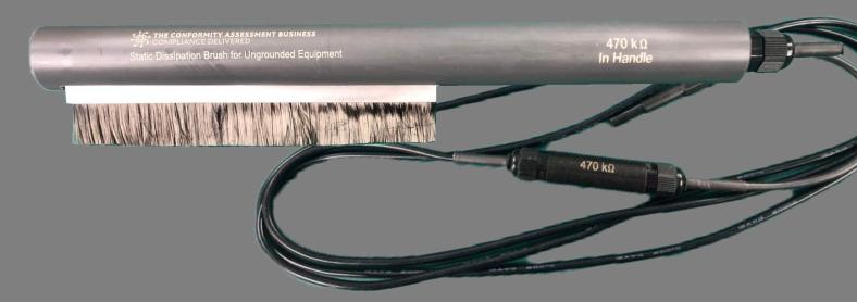
The Conformity Assessment Static Dissipation Brush is designed to meet section 7.2.4.1 of EN 61000-4-2: 2009. It is used to dissipate charge on ungrounded equipment being tested. The brush is applied to the equipment under test between successive discharges and prevents charge build up and the potential for over testing. The carbon brush is supplied with a 2m silicone cable that incorporates the required discharge resistors.
