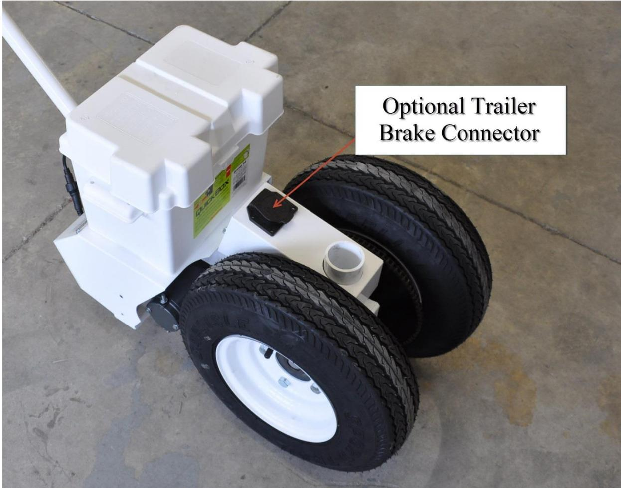
The Parkit360 Force features a connection for your trailer brake system (where the Electronic Brake Control option - extra cost - is fitted). When connected and powered on, the trailer brakes will be engaged automatically whenever the unit isn't moving. When the motor is activated, in either direction, the brakes are released automatically.
