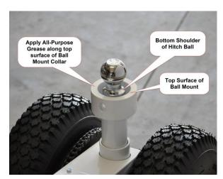
4. Using the jockey wheel, lower the trailer down onto the ball & lock it as you normally would (holding the Parkit360 level may help in this process)
