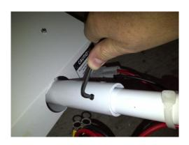
Plug in the handle control cable as shown. The cable connection is keyed, so please exercise care in making this connection.
