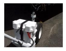
5. With pressure off the mover (using the jockey wheel), tighten the ball mount collar (counterclockwise) using the supplied tightening bar. As you tighten it, you will see the gap between the top of the Ball Mount/thrust washer and the trailer coupling close up (holding the Parkit360 level may help in this process)
