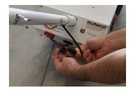
Install the Battery Box (if optioned) (using the screws supplied) WARNING - If you have the optional battery charger fitted - do not drill the screws directly above where the charger is located.
