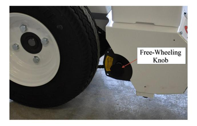
The Freewheeling knob is used to change the wheels from engaged to freewheeling mode.
