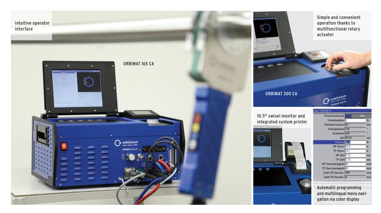
In addition to the reliable automatic programming which generates welding parameters by entering the tube diameter, wall thickness, material and welding gas all ORBIMAT CA models also include a FLOW FORCE function to reduce the pre-flow gas time when the weld heads are closed in the standard model.
