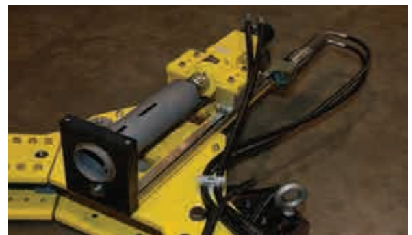
Pin drill spindle motor and feed motor operate separately
