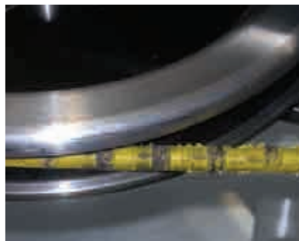
Diamond wire cutting element quickly and cleanly cuts pipe and structure of varying material and thicknesses without stalling
