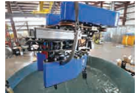
Low profile syntactic flotation package is rated for 3000msw (9843fsw)
