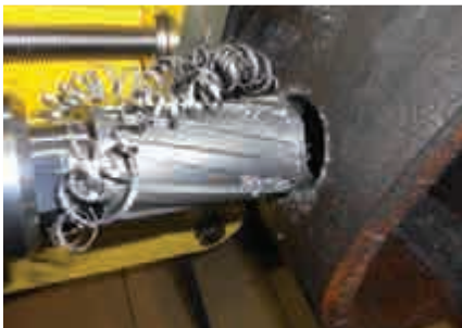
Hydraulically driven variable speed drill is powerful enough to drill a 5" (127mm) diameter hole
