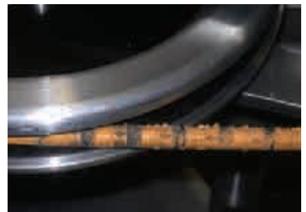
Diamond wire cutting element is easily replaced in the field, and is ideal for mixed materials and compressive cuts
