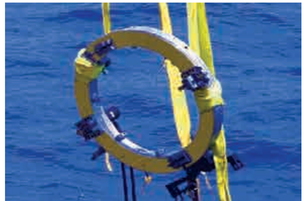
HDSF platform being lowered, note hinge for mounting
