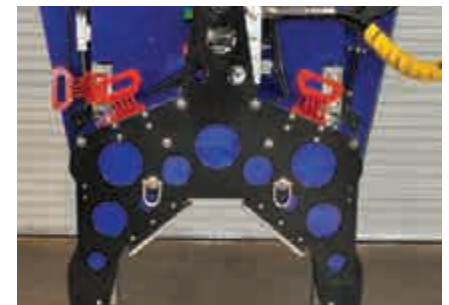
Multiple ROV compliant handles for vertical or horizontal deployment
