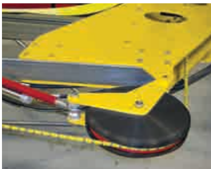
Self adjusting auto feed system controls wire tension, automatically matching the feed rate to the cutting rate
