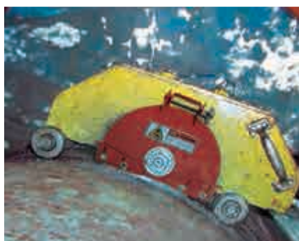
Model HE Trav-L-Cutter operates topside or subsea with its closed loop hydraulic drive system
