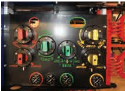
Clutched control knobs allow full control of the saw by ROV manipulation
