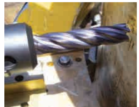
Detail of milling module which makes plunge cut before rotating on HDSF platform
